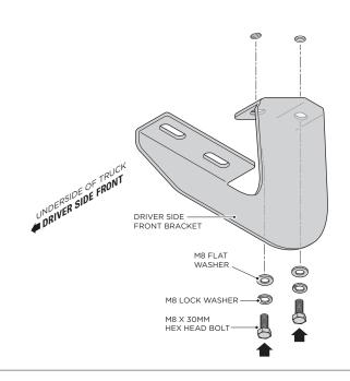
2. Fasten the Running Board to the Driver Side Front, Center Rear, Bracket cradle by using (2) M8 Flat Washers, (2) M8 Lock Washers and (2)
